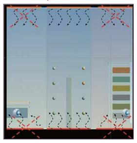
**Figure 14.7 - Probes position for comfort analysis.** Source: EPTA.
