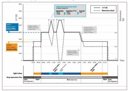
All control algorithms for luminaires include a luminous flux compensation of LED as their luminous flux depreciates over life time. At the end of life time, the luminous flux has to satisfy the predefined lighting level (design value). Without a suitable control mechanism, the LED would have a too high luminous flux at the beginning of the lifetime. Constant Light Output control CLO adjusts luminous flux accordingly over lifetime to avoid excessive light and to save energy.
