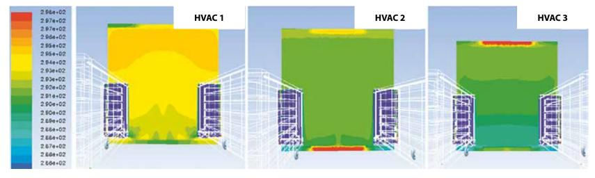
Table 14.3 reports the global and local comfort indicators calculated (by 3D Computational Fluid Dynamics simulations) using the predicted temperatures of LT and NT cabinets' zone layout. Radiant floor (HVAC 2) is more effective in reducing cold floor discomfort compared to the ceiling solution and happens to be the most energy-efficient one in winter conditions thanks to the fact that it can reach the highest PMV (Predicted Mean Vote) value among the three HVAC systems analysed.
