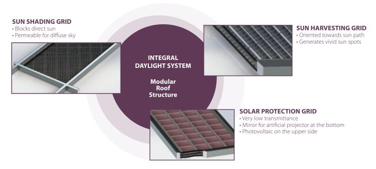
Figure 13.3 shows the sun-harvesting grid and its application in the centre fields of the sloped atrium roof in CitySyd shopping centre, Trondheim. Initially, the atrium – and as a result the adjacent restaurant – was often directly hit by sun-light at low sun angles (due to orientation of East-South-East and due to a high latitude of 63°23') causing uncomfortable glare. By applying the sun-harvesting system (which was specifically
