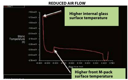
To quantify the potential advantages, 3D Computational Fluid Dynamics (CFD) simulations have been run on a freezer cabinet. Table 14 2 shows a saving of -5.25%, and max m-pack temperature close to the temperature obtained in the Class test. Following data refer to the simulated small portion of a cabinet. Without reducing the speed, the temperature lowers by 1.2°C.
