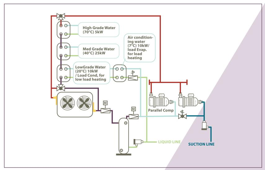
In winter conditions, the wide possibility of regulation of the high-pressure valve is able to modulate the pressure of the gas cooler. Like this, the system runs as a standard transcritical system with the possibility to actively modify the set-point of the discharging pressure, so as to modify the thermal power and temperature recovered by the heat exchanger(s).
