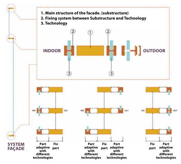
The fastening system between the main structure (substructure) and the technology must be a set of elements or parts, which achieve the fastening of the technology and establish a strong connection with the substructure. This makes it possible to define the best strategies of each situation that will be as standardized as possible.
