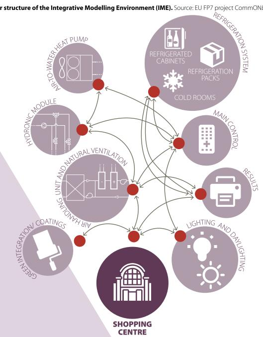
A parametric definition of the component features and the modular structure of the model layout: eases the development of a shopping centre system model, allows the optimization of the components size and the simulation of different scenarios and solution-sets, facilitates sensitivity analysis, uncertainty analysis, multi-objective optimization and model calibration.
