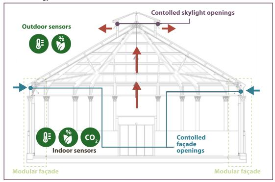
**Figure 10.4 - Interior view of the Mercado del Val with façade and skylight openings.** Source: FURAC
