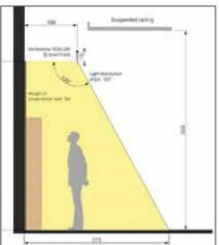
Figure 13.10 - GRL luminaire. Source: product photo and drawing from DURLUM
