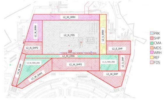
As shown in Figure 8.2 and Figure 8.3, the complex building layout is divided into 22 thermal zones, which simplifies a lot the simulation process.
